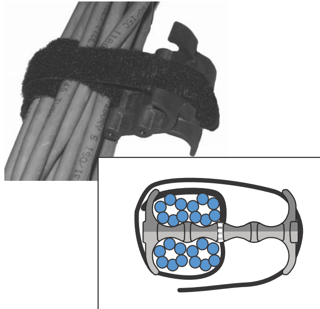
FIGURE 67 24 RJ-45 cables in four groups
